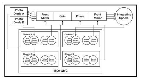
**Figure 2.** ATE system for testing four-section tunable laser diode modules. Current source cards control injection currents. Three of the four current measurement channels record photocurrents—two are for wavelength measurement, and one for recording optical output power. This testing generates from 250,000 to 1,500,000 LIV measurements. Essential ATE requirements are high channel count, multiple A/D converters, and fast transfer of large data sets to the PC controller.
